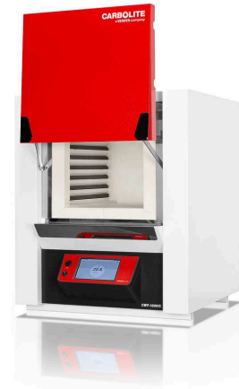
CWF 13/36 with AriesPlus temperature controller
